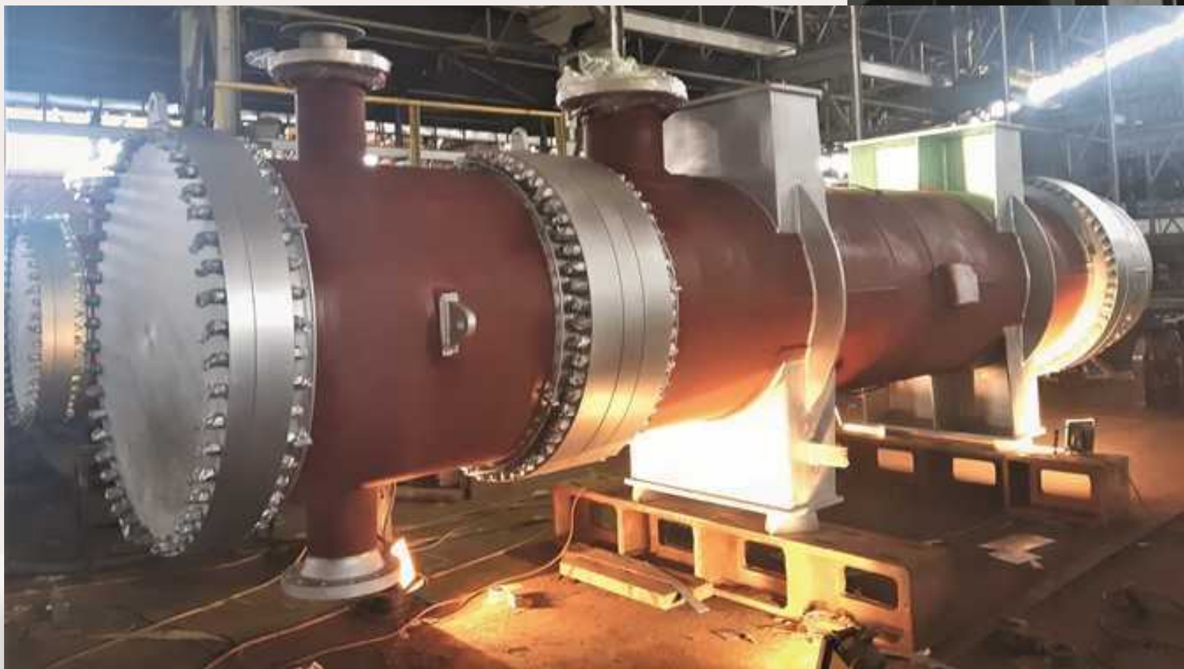
Crude / Preflash Overhead Heat Exchanger (11-E-129 A/B)
